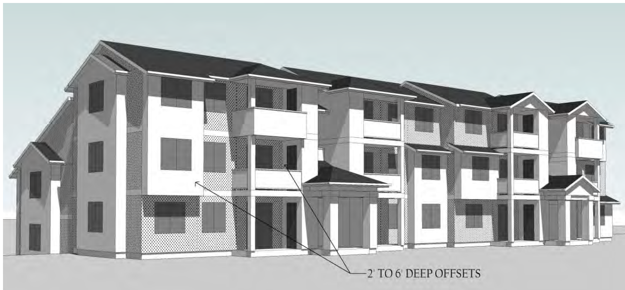
Figure 12A: Example Building Front Offset for refinement to DDH 2.E.4.b.1) as indicated in the above table
