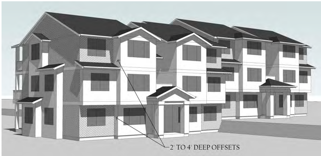
Figure 12C: Example Building Front Offset for refinement to DDH 2.E.4.b.1) as indicated in the above table
