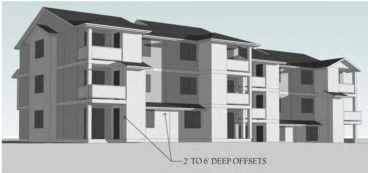
Figure 12D: Example Building Back Offset for refinement to DDH 2.E.4.b.1) as indicated in the above table
