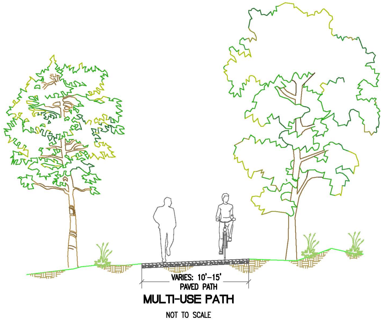
Figure 16: Conceptual multi-use path cross section
