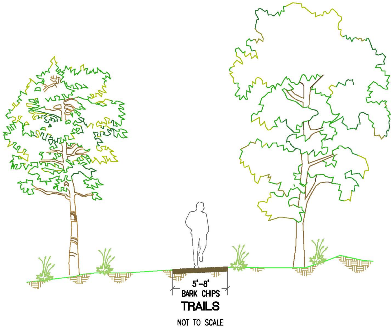
Figure 17: Conceptual trail cross section
